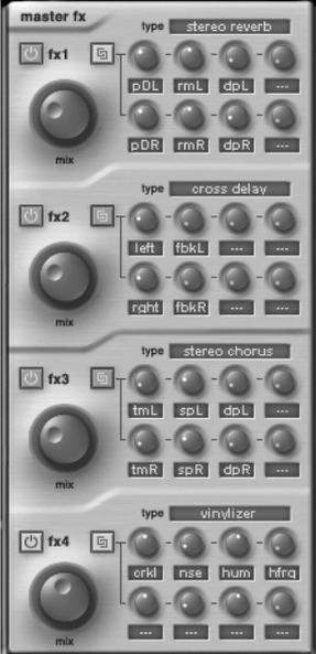
Xphrase features a Master FX section consisting of 4 separate FX processors. The four sections are routed parallel, with each assigned to a different output.
