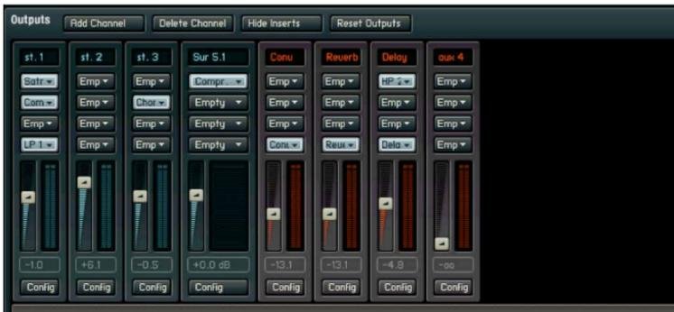
There are two types of faders: “Blue” faders that relate to channel outputs (the number of faders depends on the number of available outputs), and four “orange” faders that control return from the four send effects, as used in Multi setups. Each fader, output or aux return, has four effect insert points.
