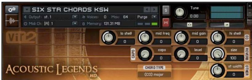
M and S buttons allow you to **mute and solo** the instrument, respectively.
