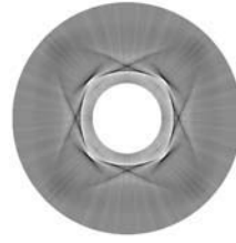
Figure 19.33. Measured normal displacement u_3(r/t, \varphi) on the surface of a copper crystal for r = 5 mm
