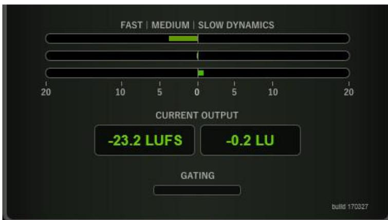
The meters are displaying the operation of all three leveling sections. There you can see how much gain or attenuation is currently happening.
