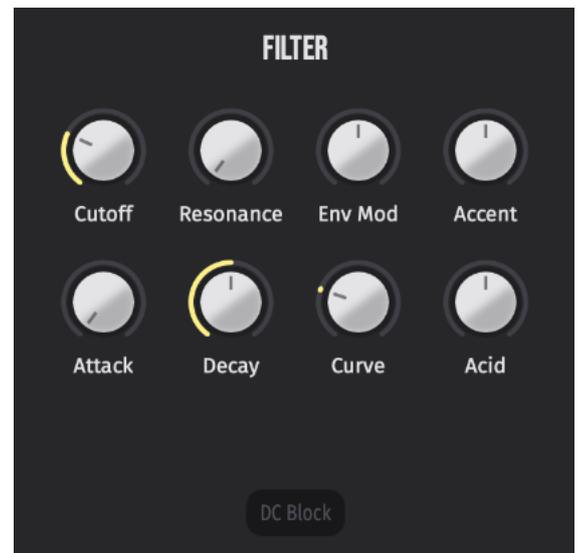
The Acid control will change the sound of the filter by altering the feedback signal within the filter circuit. **WARNING: The Acid control can cause the filter to be unstable. Small tweaks can tune the sound to your liking. But don't combine large changes with high filter cutoffs or resonances. You have been warned! ;)**
