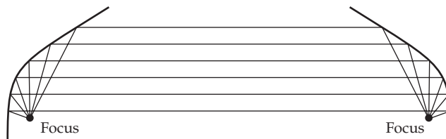
FIGURE 6-7 Graphic example of a whispering gallery showing symmetrical sound focusing points. A whisper directed tangentially to the paraboloid-shaped surface is readily heard by the receiver on the far side of the room. More generally, concave surfaces pose acoustical problems.
