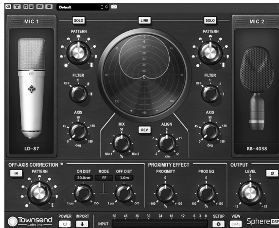
Figure 3.16 An example of a virtual mic system plug-in, used to select the model, polar pattern, orientation, and other characteristics of the mic being modelled. This screenshot shows the plug-in in “dual” mode, where the single (dual diaphragm) virtual mic simultaneously models two different mics.
