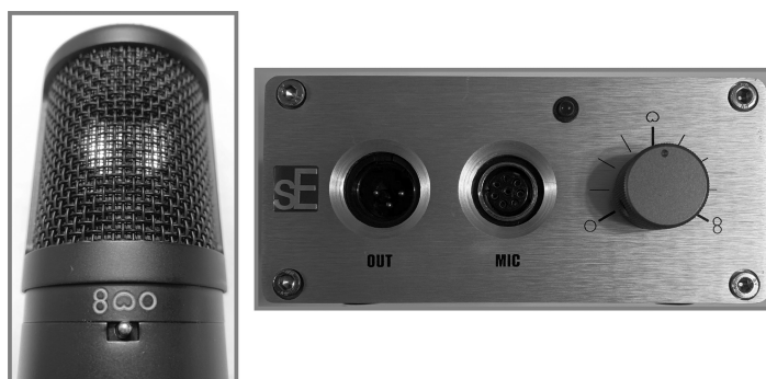
Figure 3.11 Left: A three-pattern selection switch on a multi-pattern microphone. Right: A rotary switch on an external (tube mic power supply) box allows selection of a variety of intermediate pick-up patterns.
