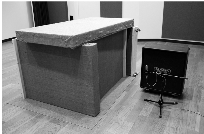
Figure 10.8 The guitar speaker cabinet and its mic (in the right of the picture) can be placed inside a “cage” of homemade gobos (in the left of the picture) to isolate it from the room and reduce its spill into any mics set up on other sound sources in the room.
