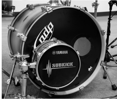
Figure 3.17 A commercial loudspeaker cone mic on a kick drum.
