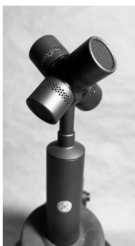
Figure 8.7 A First-Order Ambisonic mic with a tetrahedral array of cardioid capsules.
