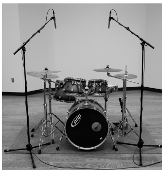
Figure 12.5 A spaced array with a mic positioned over each bank of cymbals, at the first and third “quarter” divisions of the width of the set.
