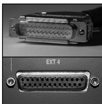
Figure 1.26 25-pin D-Sub connectors. Top: Male. Bottom: Female.
