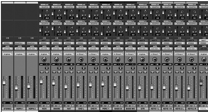
Figure 18.1 Two headphone monitor mixes in a DAW. Two stereo sends (the top two small faders of each channel) are assigned across all tracks, with different mixes (amplitude and panning) dialed in for each. On the left of the mix window are the master faders for the main stereo mix, and the two headphone mixes.
