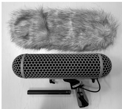
Figure 19.4 A blimp and pistol grip system. The microphone attaches to a shock mount inside the blimp, which is attached to the pistol grip. This pistol grip can be attached to a boompole, or hand-held. The blimp can be removed from the shock mount for indoors, no-wind situations. The dead cat windscreen can be stretched over the blimp in windy conditions.
