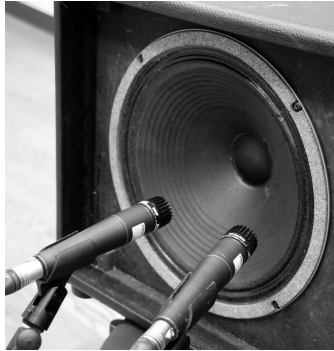
Figure 14.1 A guitar cabinet loudspeaker miked on-axis for the brightest sound, and off-axis for a warmer sound.
