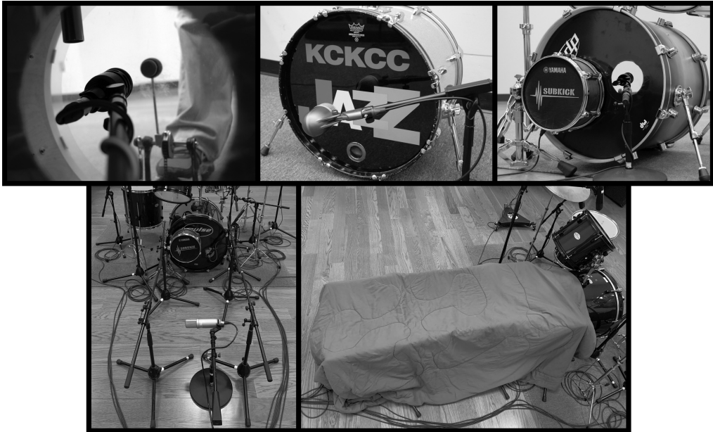
Figure 12.1 Top Left: Looking through the hole into a kick drum with a mic typically placed for single mic recording, several inches from the beater-side head. Top Center: A mic about 15 cm (6 in) outside the center of a jazz kick drum. Avoid miking at or close to the outside of a hole as small as the one in this drum – a very strong air current is forced through a hole this small. Top Right: A combination of a loudspeaker cone mic, and a conventional mic inside the drum. Bottom: An additional mic is placed several feet from the kick drum, and comforters, duvets, blankets or whatever is on hand is used to isolate it from excessive spill in a “tunnel.” Short mic stands are used here, in “T” formation, to support the blankets.
