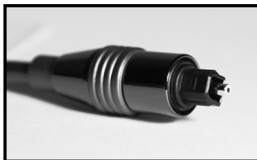
Figure 1.27 A TOSLINK optical fiber connector as used for optical SPDIF connections, and ADAT Lightpipe connections.
