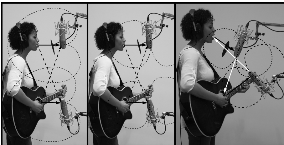
Figure 11.2 Left: A singer/guitarist miked with cardioid mics. Each mic picks up significant off-axis spill. Center: Using bidirectional mics on-axis to their desired sound source does not maximize rejection of spill. Right: The null points are aimed at the sources of spill, while keeping each mic on-axis with their desired source.
