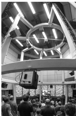
Figure 8.8 Left: A simple 3D Ambisonic loudspeaker set up, the grey balls represent loudspeakers pointed towards, and equidistant from, the listening position in the center of the cube. The front center of the soundfield is in the center of one of the “walls.” Right: A 33.2 dome with five layers (4, 8, 8, 8, 4+1, floor to top), used for higher-order Ambisonic work (Hamburg University of Applied Sciences, Germany).
