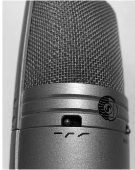
Figure 4.5 A low cut filter switch on a mic.
