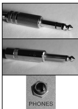
Figure 1.23 Top: A quarter-inch TRS male plug. Middle: A quarter-inch TS male plug. Bottom: A quarter-inch female socket/jack (it could be TS or TRS – there’s no way to tell visually, but “Phones” here indicates that it is TRS).
