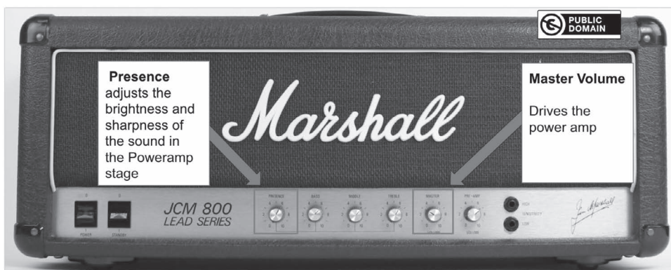
Figure 3.9 The power amp stage is controlled by the master volume and presence knobs.
