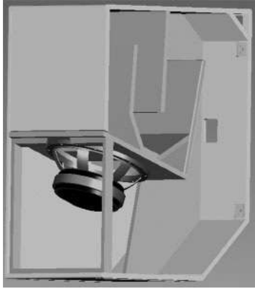
Figure 21-33. Tapped Horn™ cutaway.
