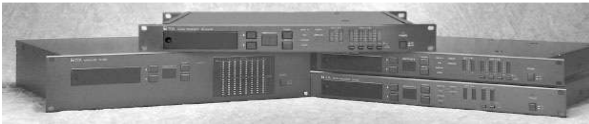
Figure 41-3. TOA Dacsys II digital audio processors (center and right). TOA's second generation digital audio processor (the SAORI was the first), it had a Windows-based control program, which allowed a limited amount of internal reconfiguration of the signal flow. On the lower left is a digitally controlled analog matrix mixer, which could be controlled with the same program.
