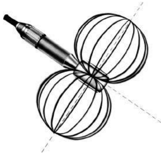
Figure 20-12. Bidirectional pickup pattern. Courtesy Sennheiser Electronic Corporation.
