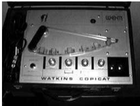
Figure 28-12. Tape loop delay system.
