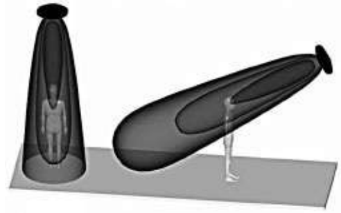
Figure 44-18. Mounting angles for Audio Spotlight systems. Courtesy Holosonic Research Labs, Inc.
