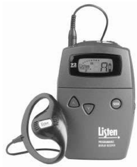
Figure 44-15. Typical high-quality FM receiver, the Listen LR-500-863. Courtesy Listen Technologies Corporation.
