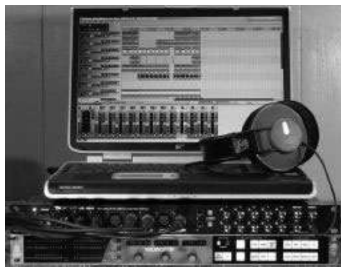
Figure 29-138. A modest-sized DAW running on a USB link between the audio interface unit (center) and the laptop. The (almost free) DAW software allows for 48 simultaneous recorded tracks, with significant audio processing. Complete with shown external mic-amps and computer, the cost of this outfit is about that of a decent microphone; its 1990 equivalent in facilities and performance would have cost the same as a decent car, while the
