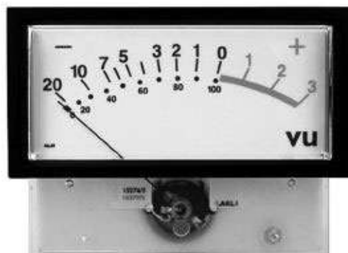
Figure 30-1. Moving coil VU meter.
