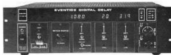
Figure 41-1. Introduced in 1974, the Eventide Clockworks Model 1745M modular digital audio delay was the first to use random access memory (RAM) instead of shift registers for storage of sound. Options included pitch changing and flanging.
