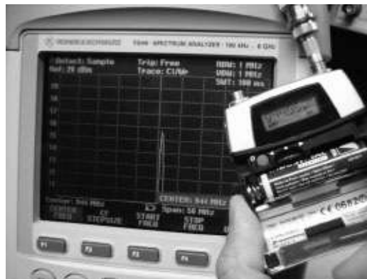
Figure 20-172. Sennheiser SK 5212 bodypack transmitter and a spectrum analyzer. Courtesy Sennheiser Electronic Corporation.
