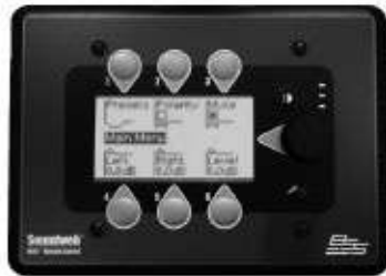
B. BSS Audio Soundweb 9010 Remote Control. This is an example of a dedicated remote control panel that may control internal Soundweb controls. Six buttons, a rotary encoder, and a LCD display are provided.
