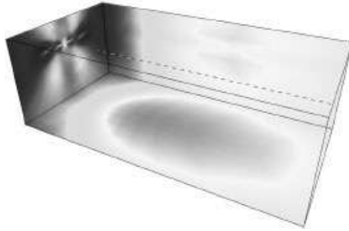
Figure 38-8. Direct field map of audience area in room model (CATT-A).
