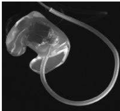
Figure 4-14. Close-up of custom in-ear monitor showing balanced-armature drivers. Courtesy Sensaphonics.
