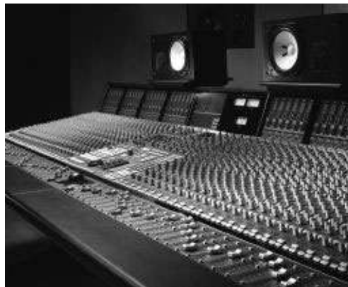
Figure 29-101. SSL AWS – an analog music tracking console. Courtesy Solid State Logic.
