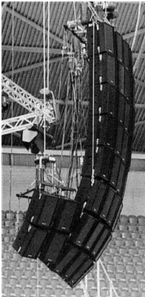
Figure 22-1. A typical second generation loudspeaker cluster. Even when a single enclosure is designed to resemble a point source, multiple enclosures will always interfere with each other when connected to a coherent audio signal.
