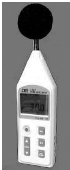
Figure 49-1. A sound level meter is basically a voltmeter that operates in the acoustic domain. Courtesy Galaxy Audio.
