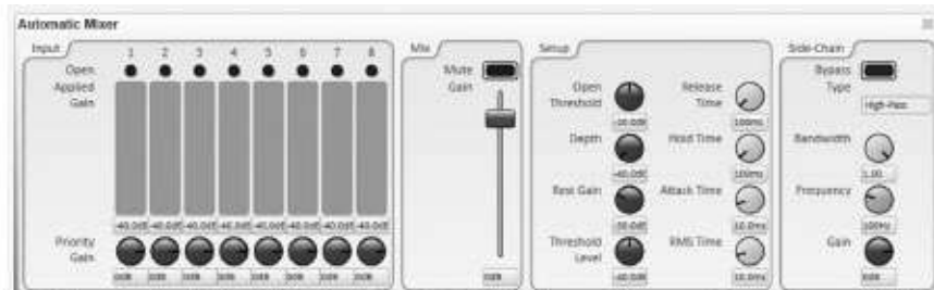
A. Inside a typical Virtual Device from QSC. This shows the sort of controls and indicators found inside the Virtual Devices in Fig. 41-7.
