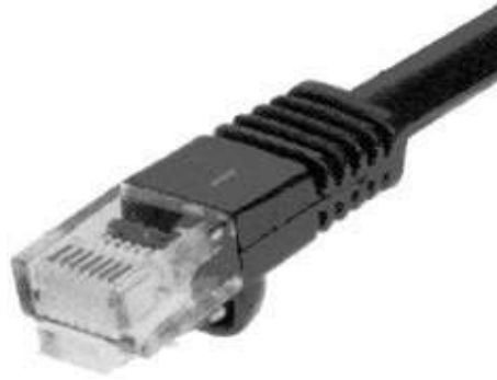
Figure 42-32. “RJ-45” plug. This is an 8 position 8 contact nonkeyed modular connector originally developed for telephone applications. It is the connector used for all UTP cables in Ethernet networks.
