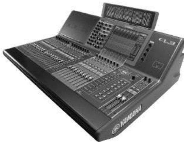
Figure 41-2. The CL3 Digital Mixing Console from Yamaha is part of a family of audio mixers. The size of the mixer has no direct relationship to the number of audio inputs and outputs controlled. The audio input and output connections are in stage boxes that connect to the console via a Dante network. If desired a separate mixer can be used for monitor mixing yet share the same input connections.
