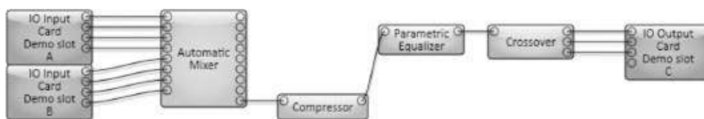
Figure 41-7. A simple example of a virtual sound processor schematic from QSC Q-Sys.
