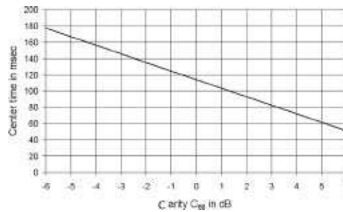
Figure 9-17. Center time t_S as a function of the clarity measure C_{80} .
