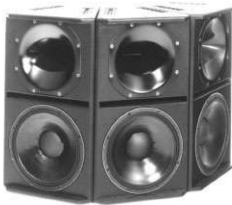
Figure 22-12. TRAP arrays can be quite small; however, the size of the horns will determine the lower frequency limit at which the True Array Principle ceases to operate.
