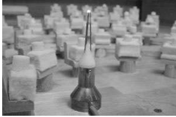
Figure 13-4. A spark generator used in scale physical models. Courtesy Kirkegaard Associates.
