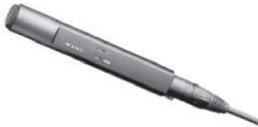
Figure 20-71. Omnidirectional pressure capacitor microphone. Note the lack of rear entry holes in the case. Courtesy Sennheiser Electronic Corporation.
