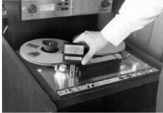
Figure 32-30. Tension measurement. Courtesy Ampex Corp.
