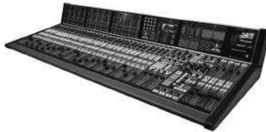
Figure 29-139. The Wheatstone Dimension 3 large-format TV audio console, a control surface which has no audio in it at all! It merely controls a remote mixing router, and connects with its I/O via either UDP or AoIP.
