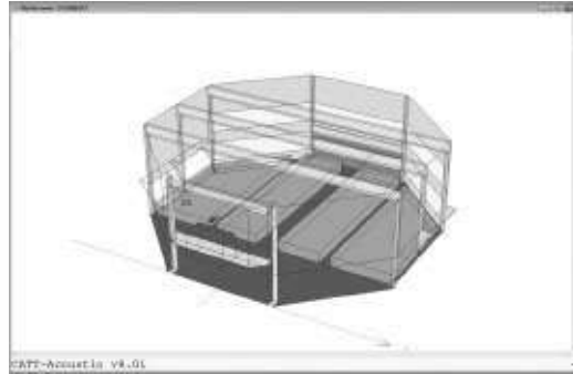
Figure 38-10. The wire frame room model provides a virtual design environment (CATT-A).
