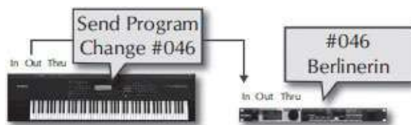
Figure 33-12. Program Change messages can be used to change sound patches from a sequencer or from a remote controller.
