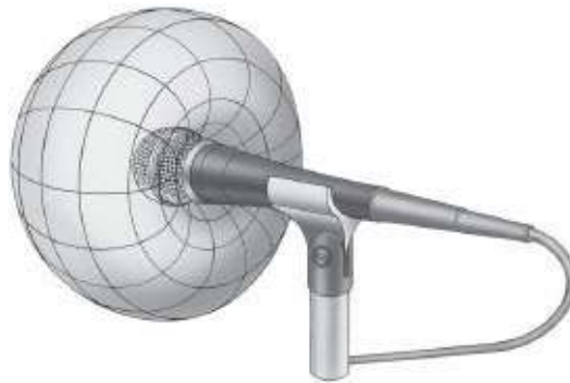
Figure 20-14. Cardioid pickup pattern. Courtesy Shure Incorporated.
