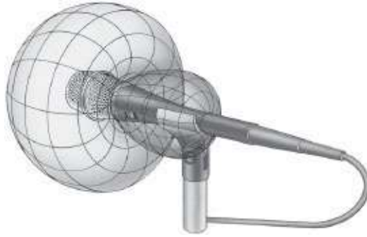
Figure 20-15. Supercardioid pickup pattern. Courtesy Shure Incorporated.
