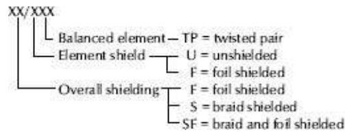
Figure 18-3. ISO/IEC 11801 cable naming convention.
