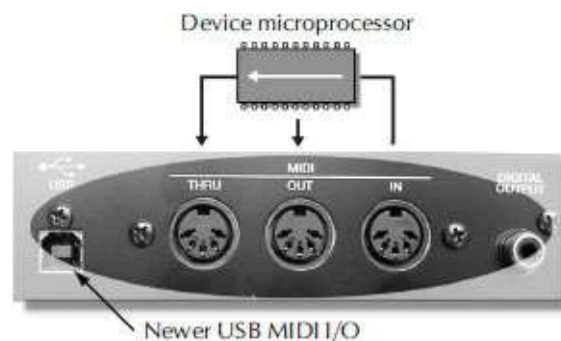
Figure 33-3. MIDI In, Out and Thru ports, showing the device's signal path routing.
