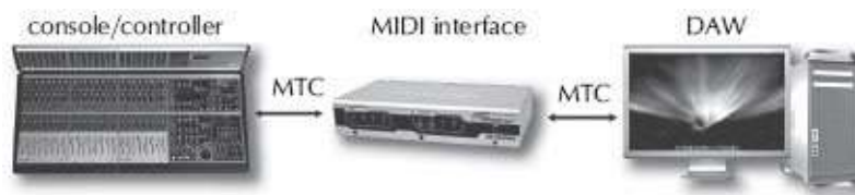
Figure 33-27. Many time-based media devices in the studio can be cost effectively connected via MIDI timecode (MTC).
