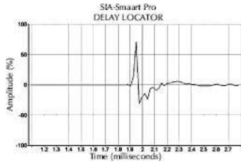
Figure 49-29. The impulse response of a transducer with correct polarity.
