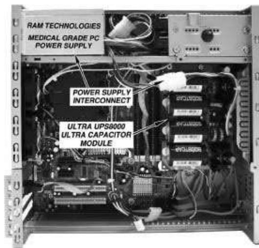
Figure 23-35. Typical installation of a ultracapacitor UPS module in a computer. Courtesy Ram Technologies LLC.
