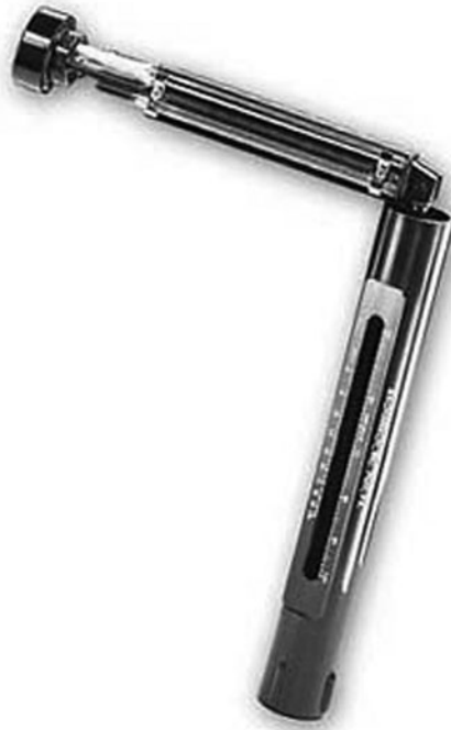
Figure 7.2 A typical sling psychrometer.
