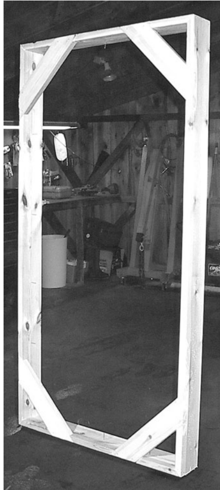
Figure 9.2 Fiberglass panel frame.
