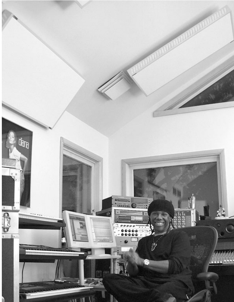
Figure 9.31 MiniTraps in Nile Rodgers' control room 11 .
