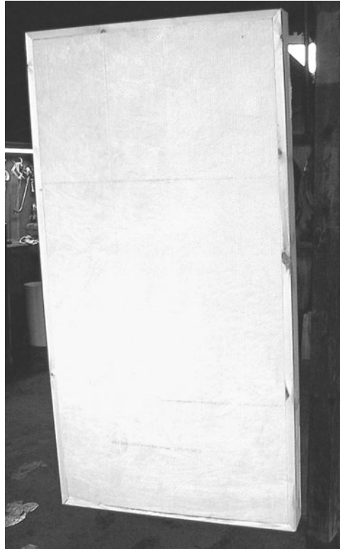
Figure 9.3 Fiberglass panel—frame with insulation.
