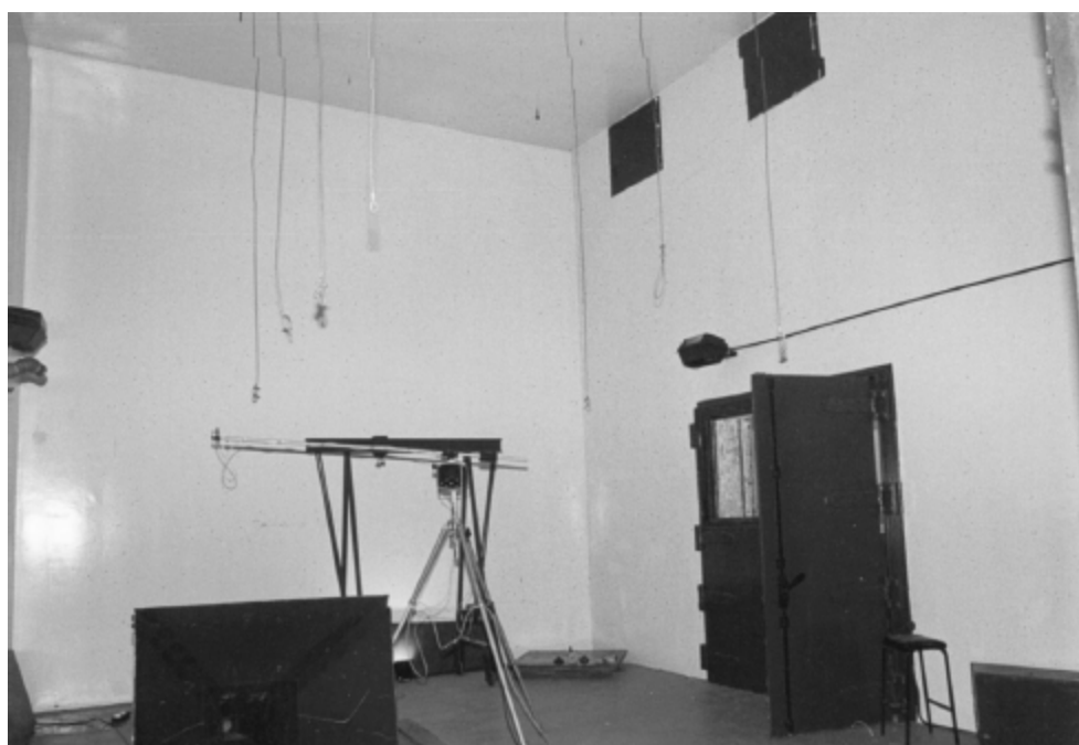
Figure 4.1: The large reverberation chamber at the ISVR. It has a volume of 348 \text{ m}^3 with a reverberation time of 10 s at 250 Hz, and 5 s at 2500 Hz. All surfaces are non-parallel and are made from painted concrete.
