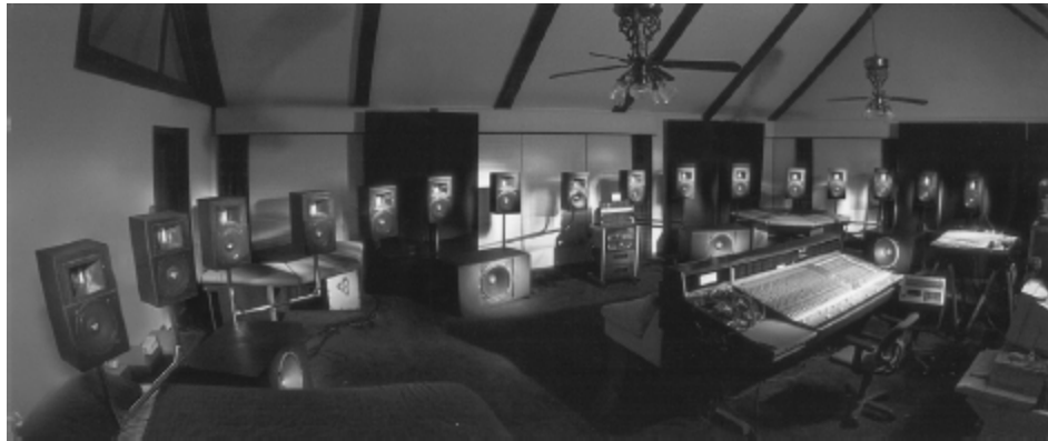
Figure 19.20: The multi-channel monitoring system in the private studio of Eugene Czerwinski, the founder of Cerwin Vega Inc. The use of one-track-to-one-monitor is said to reduce drastically the levels of intermodulation distortion, and to increase greatly the level of perceived openness and neutrality in the reproduced sound (photograph courtesy of Eugene Czerwinski).
