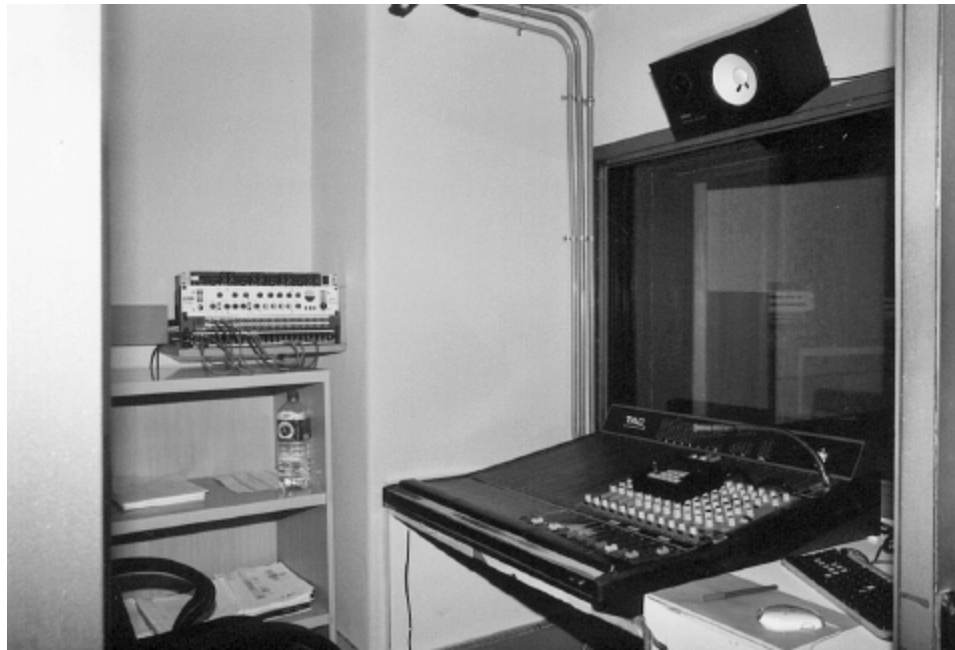
Figure 5.28: An absurdly small 'control booth'. Rooms of such small sizes are effectively too small to allow a flat monitoring acoustic, and colouration is unavoidable.
