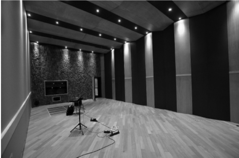
Figure 6.18: The large Foley-stage at Loudness Films, in Lisbon, Portugal; completed in 2014. It has different surfaces on different walls, to allow recording in areas with different natural acoustics.
