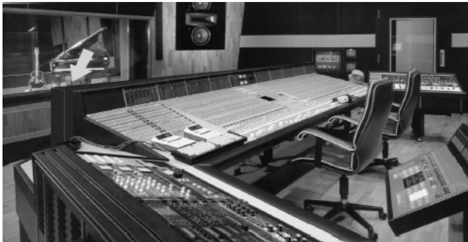
Figure 18.1: Acoustic screen to suppress console reflexions (indicated by the arrow). A freestanding screen can be mounted behind the mixing console, spaced away by 15–20 cm to allow free ventilation if necessary. The screen should be around 20 cm thick,
