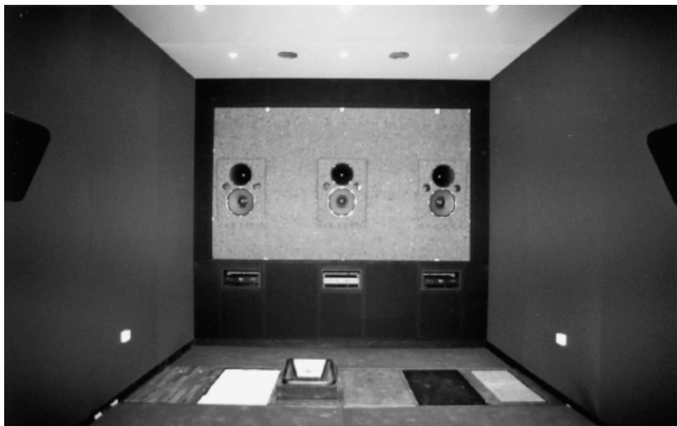
Figure 6.15: The Foley room at Cinemar Films, Milladoiro, Spain, with the perforated screen dismantled and the different walking surfaces clearly visible. This room, with a mixing console installed, can also be used for pre-mixing ‘stems’ of dialogue, music or effects, hence the surround loudspeakers which are visible at each side of the photograph (2006).
