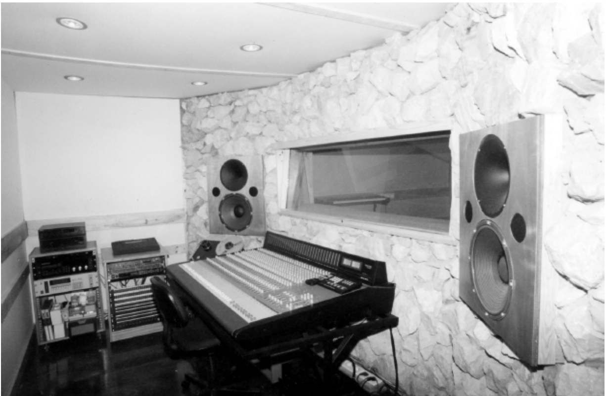
Figure 16.9: A very small Non-Environment control room: Noites Longas, Redondos, Portugal. The room was built in a shell of only 3m×4m, with a sloping roof, but the acoustic situation was helped
