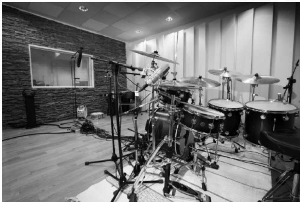
Figure 7.11: Drum room with variable acoustics by means of narrow, hinged panels and movable ceiling tiles. Mikeal Wikman Drum Studio, Stockholm, Sweden (2012).
