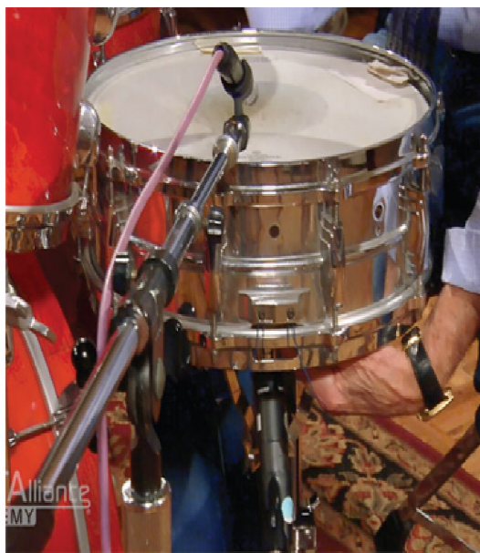
AKG C452 on the top snare head and a Shure SM57 on the bottom.
