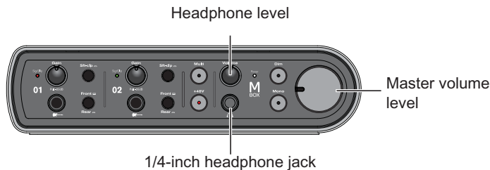
Mbox front panel connectors and controls
