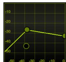
Compressor settings can be initialized efficiently by using one of the preset curves (accessible via the small drop-down menu in the upper-left corner). This menu also allows you to copy curves from one equalizer/dynamics processor section to another.
