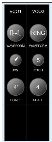
Figure 7: The MS20 oscillators producing an enharmonic timbre.
