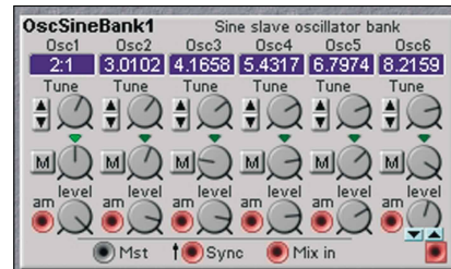
Figure 9: Generating a stretched spectrum comprising six partials.
