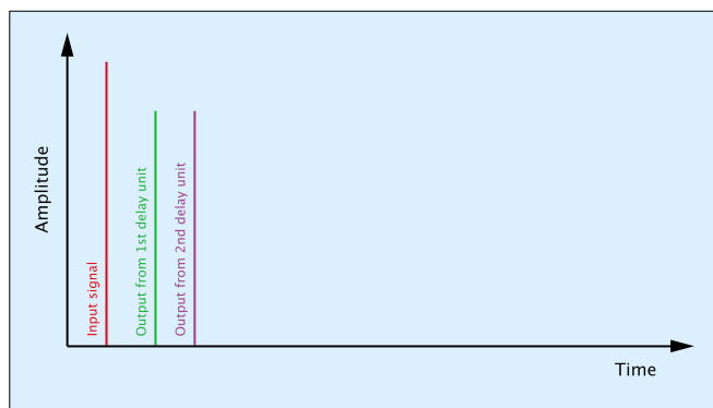
Figure 13: Two delays without regeneration.
