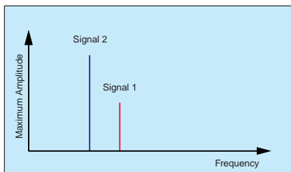
Figure 7: The harmonic spectrum of the mixed signals.
