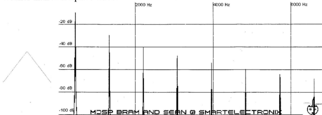
Figure 8. A triangle wave has odd harmonics that are weaker than those of a square wave.
