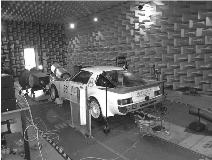
Figure 24.3: Sweep recording on the Motor Industry Research Association's “rolling road” chassis dynamometer
