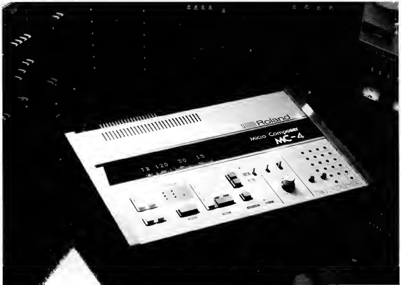
Fig. 3-32 Roland MC-4 MicroComposer (Computer Controller)
