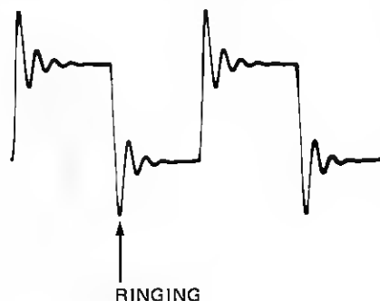
Fig. 3-19 Effect of VCF resonance on square wave
