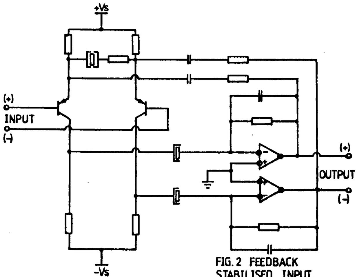
FIG.2 FEEDBACK STABILISED INPUT.
