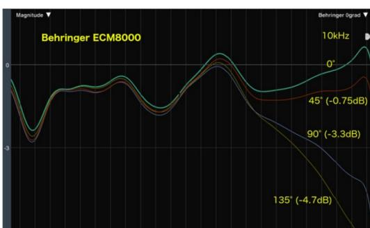
At 8kHz the differences between 0 degrees and 90 degrees range between 1.3dB for the EMX-7150 and 2.7dB for the ECM8000. At 10kHz the deviation grows to 3.3dB, at 12kHz to 4.0dB with the ECM8000, and with the EMX-7150 1.75dB at 10kHz and 2.2dB at 12kHz.
