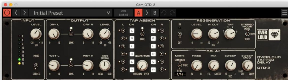
**INPUT LEVEL** - Controls the level of the **INPUT** signal.
