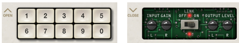
Hidden Controls with panel closed (left) and panel open (right)
