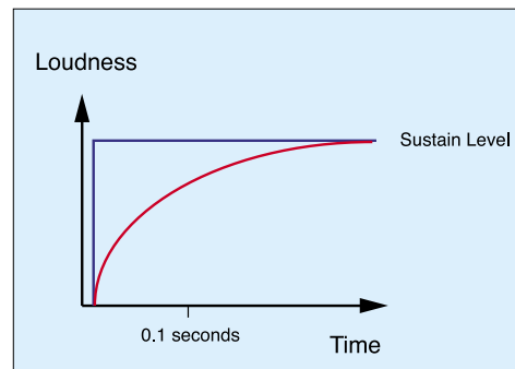
Figure 3: The real response of an ADS circuit.
