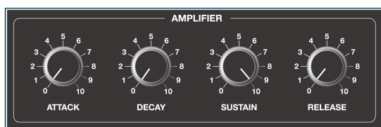
Figure 9: The 'organ' amplitude envelope settings.
