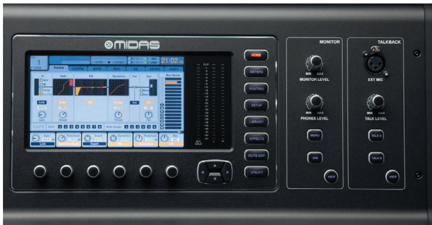
The buttons at the right select the control block that is shown on the display. The buttons/controls on the bottom of the display are used for navigation.
