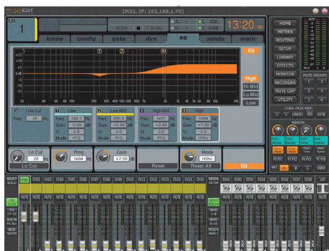
ill. 1: Overview of the external editor software: EQ window selected, all the filter parameters and the resulting curve are displayed
