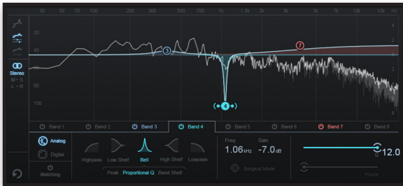
Figure 1: a narrow filter (Q=12)
