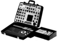
The Synthi AKS (my first synthesizer) is basically a VCS3 repackaged in a neat plastic suitcase together with a revolutionary velocity-sensitive touch keyboard cum realtime sequencer - the KS.
